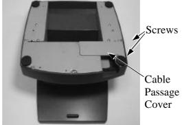
Now, unscrew the 2 screws on the cable passage cover and take the cable passage cover away to show the cable passage.
